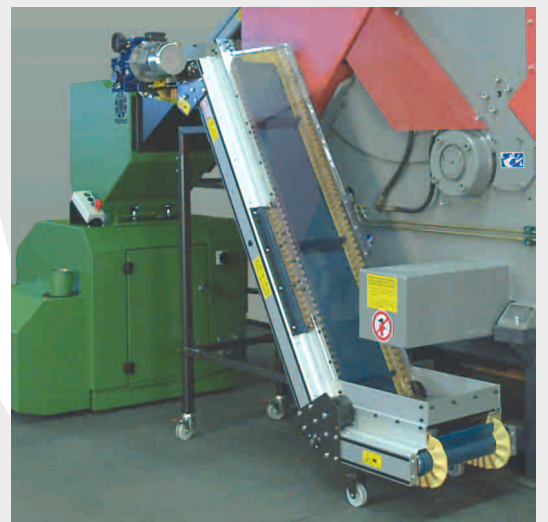
2036 with elevator conveyor for automated infeed and compact foot print.
