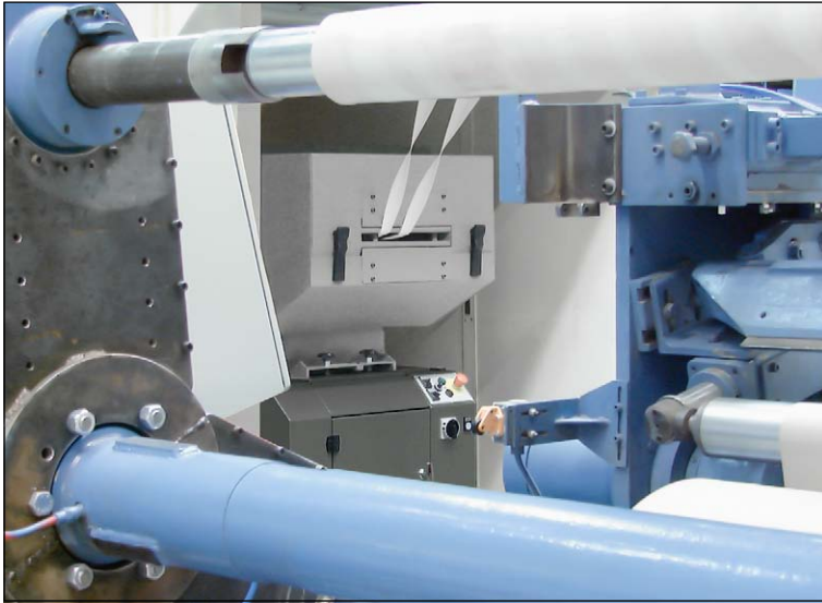
Rapid 2036 "KURF" granulator with RFL-30 infeed for in line recycling of extrusion edge trimmings.
