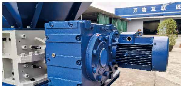
两台独立电机驱动加上高安全系数减速机产出超高扭矩。 Two independent drives with gear reducers bring a high torque.
