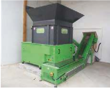
Shredder EZ 8/2 installed in a pit. Material transport by a 11 meters ascending worm screw going up to silo filling.
