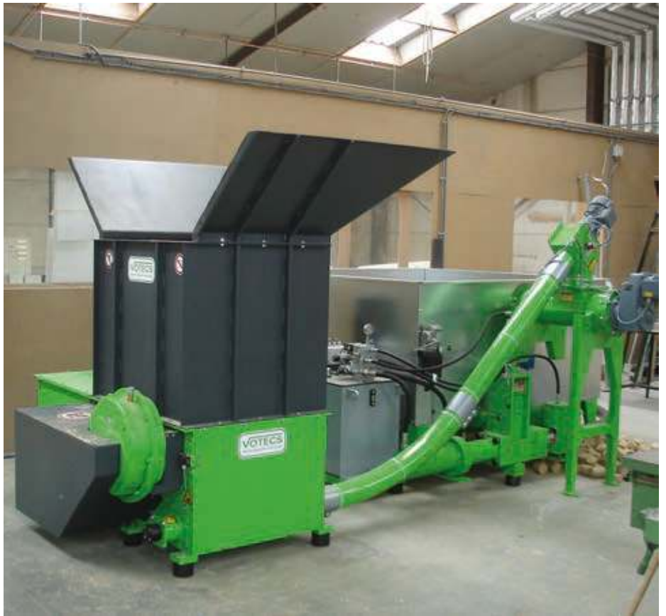
Left: EZ 10/2 , Power 37 KW, Filling with scrap wood via the conveyor belt, material discharge via a screw to the slate floor conveyor.
