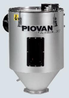
Hoppers from the T30 to the T400 (the number indicates the capacity in dm<sup>3</sup>) have a 60mm insulation layer. From the T600 up, the insulation layer is 100mm thick.
