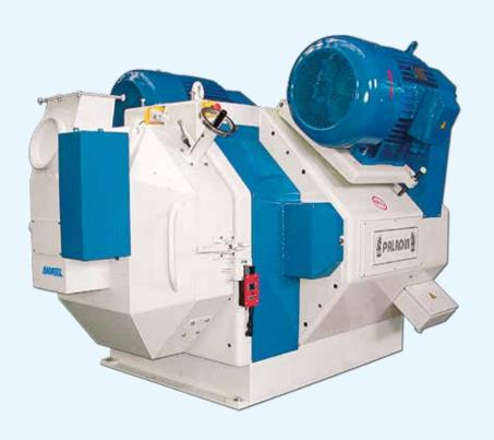
The authentic and sturdy Paladin design is constructed with a balanced twin drive system, where the transmission consists of a combination of V-belts and a toothed belt. The design of the main shaft and rotor allows maximum torque to be applied in the pelleting section. These features make the Paladin pellet mill range universally adaptable machines, en-
