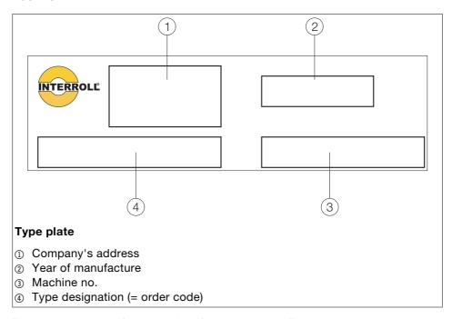
The type plate specifications identify the conveyor. The type designation is required for correct application of the conveyor.
