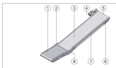
Design of type for inclined or declined belt conveyor with power feeder/outfeeder belt type 4081.8
