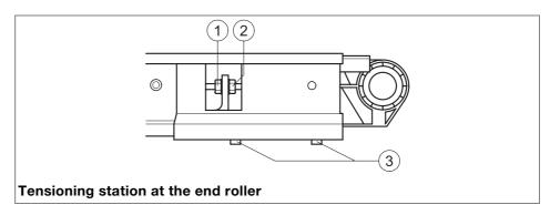
Never loosen the fastening screws (3) at the tensioning console!
